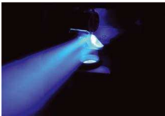
Picture 10: The blue laser with a wavelength of 405 nm
